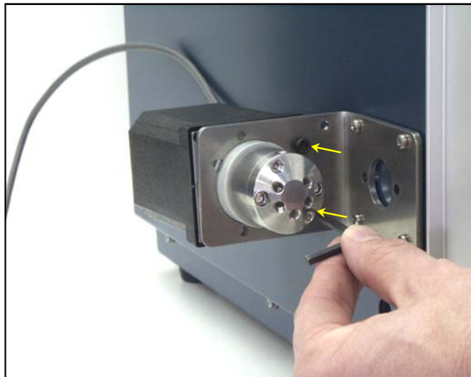
Figure 9. Securing valve in external valve bracket.
